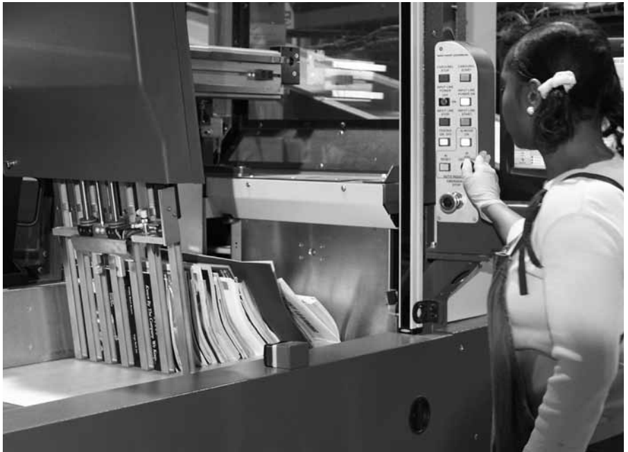
The Flats Sequencing System (FSS) automates the placement of larger mailpieces in the order in which they are delivered, which reduces the time carriers need to prepare the mail for delivery.
