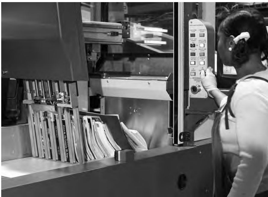
The Flats Sequencing System (FSS) automates the placement of larger mailpieces in the order in which they are delivered, which reduces the time carriers need to prepare the mail for delivery.
