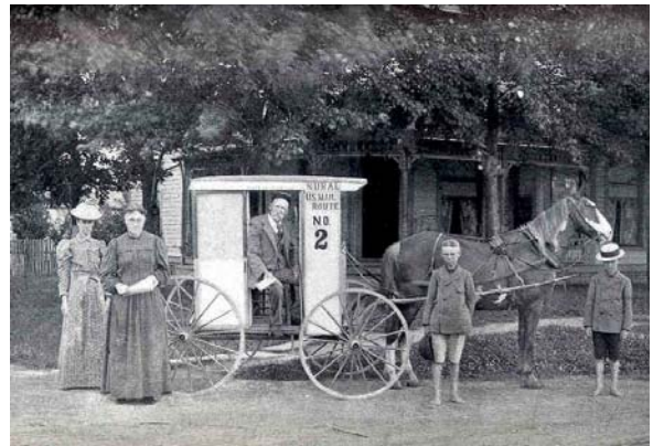
One-horse RFD wagons were manufactured and sold by private distributors for approximately $45. They came complete with sliding doors, windows that could be opened and closed, pigeonhole letter cases, a "desk" surface, and a cash-and-stamp drawer with lock and key.
